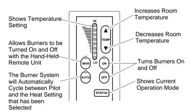
Figure 58 - Hand-Held Thermostat Remote Control Unit Selections (CGHRCT Only)
